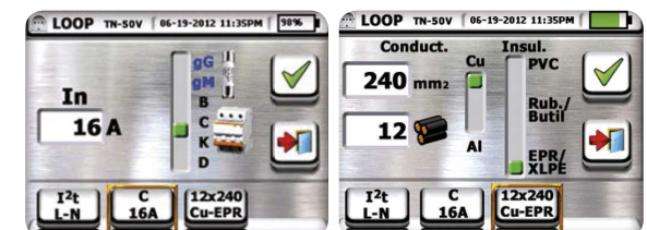
Setting of MCB/fuse type and rated current
